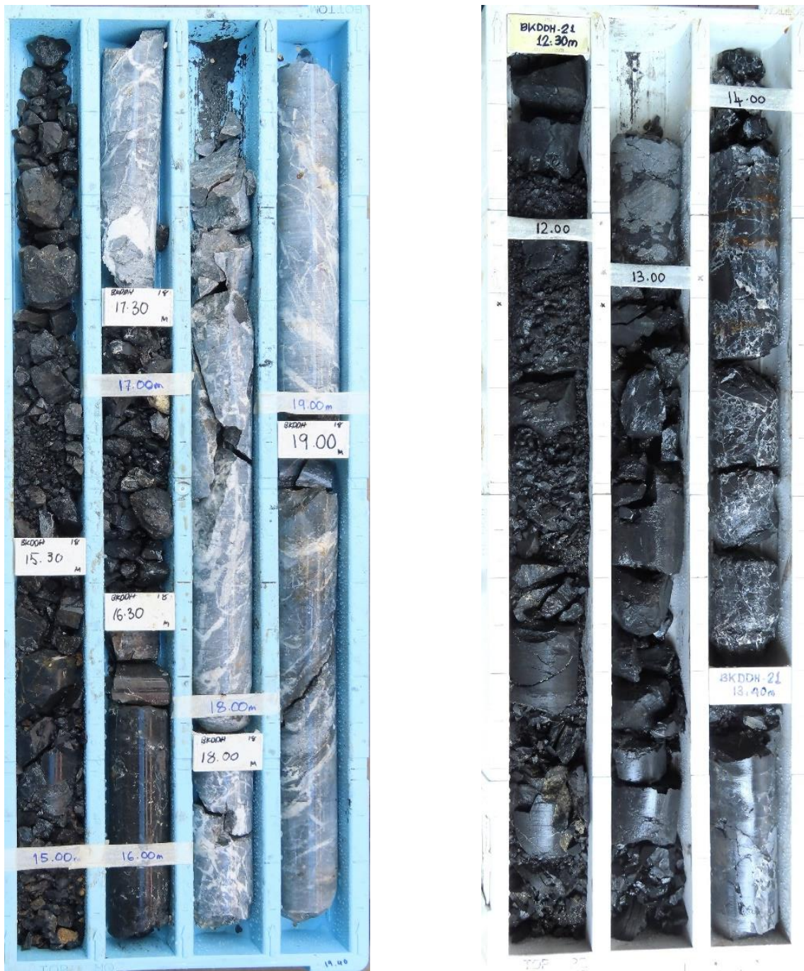
Figure 5: Examples of hydrothermal alteration involving intense calcitic, siliceous and sulphide veining and stockworks at BKDDH-18 (LEFT) within the upper Bau Limestone, near the boundary with the overlying Pedawan Formation shales (approx. 16m sub-surface). Brecciation and similar alteration textures are observed within the overlying Pedawan Formation, above the Bau Limestone contact, in BKDDH-21 (RIGHT). Historical drilling indicates that these textures are associated with sulphide endowment and gold, silver, and base metal mineralisation.
