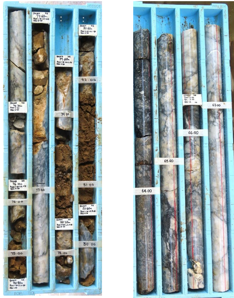
Figure 11: Section BKDDH-25 (LEFT), illustrating the intimate relationship between clay infill and karstic texture within the Bau Limestone at ~75m depth. Surrounding limestone is fractured and extensively stylolised with dark sulphides. BKDDH-26 (RIGHT) shows hydrothermally brecciated and stylolised textures in Bau Limestone at 63m – 67m depth
