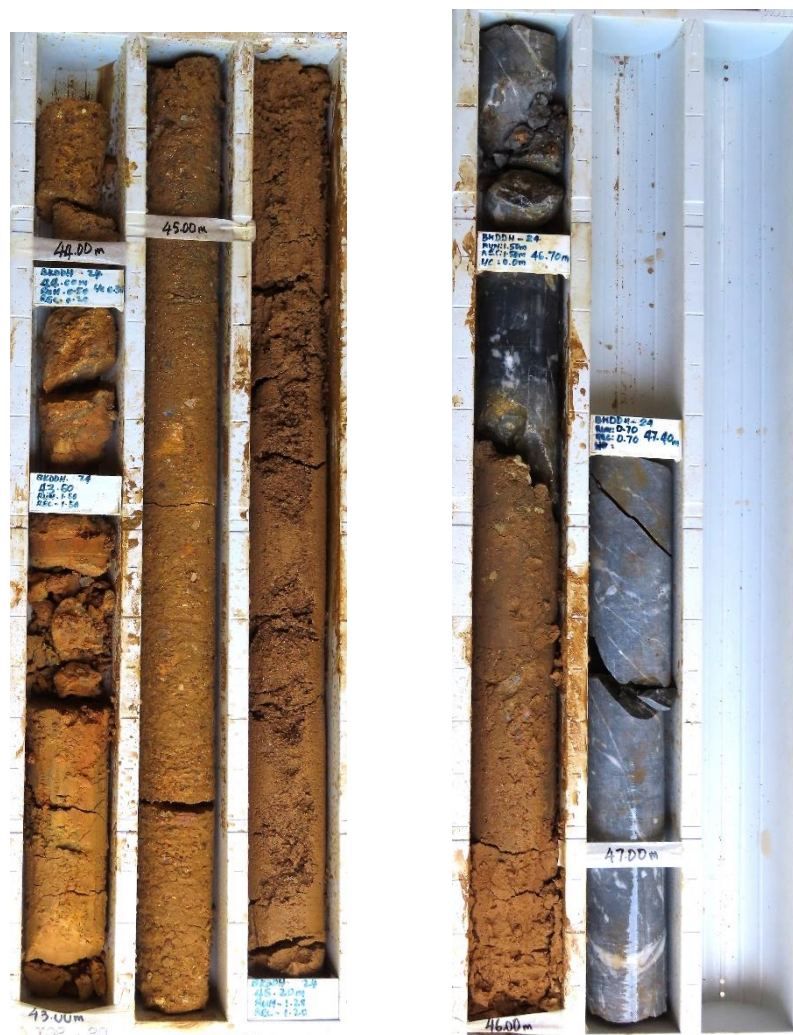
Figure 10: Section BKDDH-24, illustrating the highly weathered (oxidised) clay dominated lithologies extending from the surface to the top of the Bau Limestone, at a depth of 47m in BKDDH-24.
