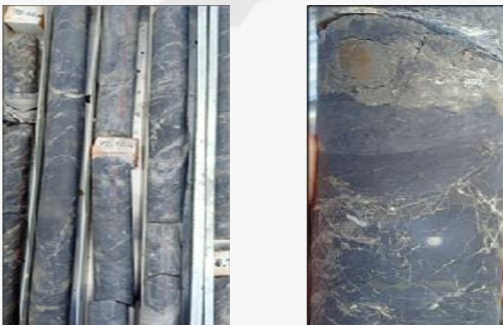
Figure 1: (Left) Drill core showing typical sulphide related mineralisation within veining at JUDDH-89 core. (Right) Close-up of a more intense zone of sulphide mineralisation in JUDDH-90 – assay results pending for both.
