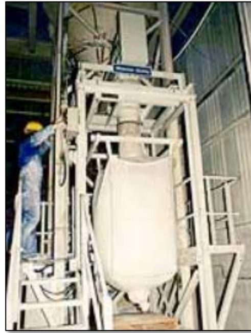
Figure 24-35 - Mechanised Fill System
