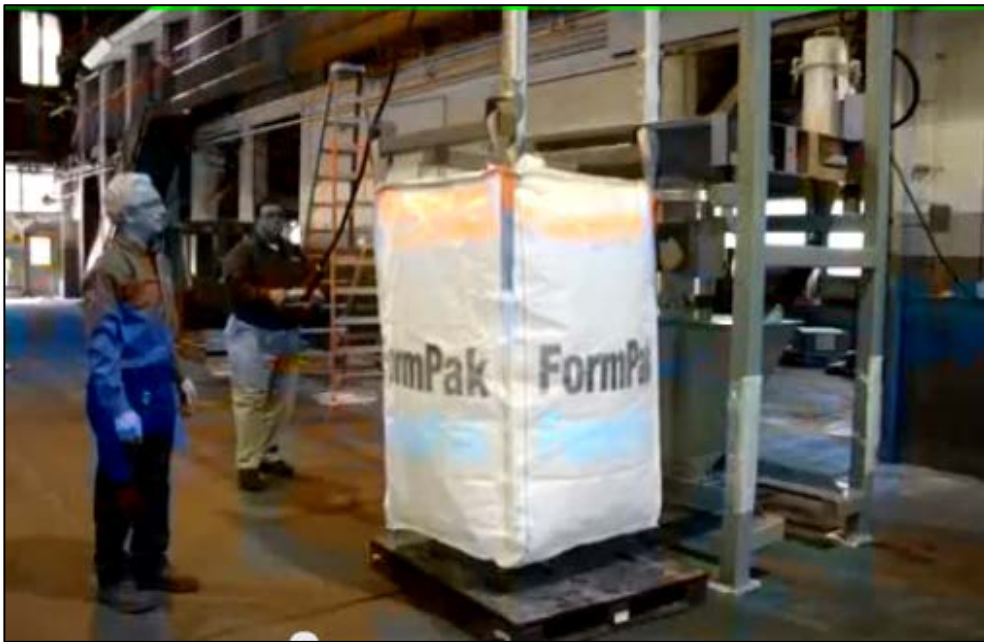
Figure 24-38 - Loading / Unloading using Overhead Trolley
