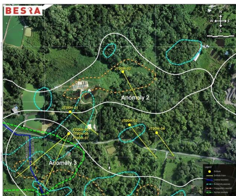
Figure 8 - Drilling locations within the 2023-2024 Exploration DDH Program. Chargeability (red polygons) and Resistivity (blue polygons). HyChips anomaly (yellow polygon) and 450hz DIGHEM resistor (dashed orange outline).
