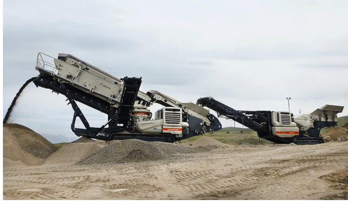
Figure 2: Example of In-pit Two Stage Crushing
