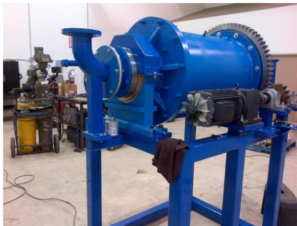
Figure 3: Example of Pilot Plant Rod/Ball Mill
